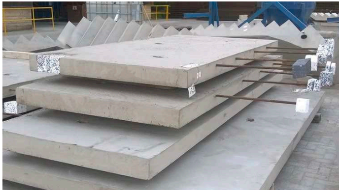
Figure 10 – Simple RC slab with cast in bars for tying back to the main floor slab.
